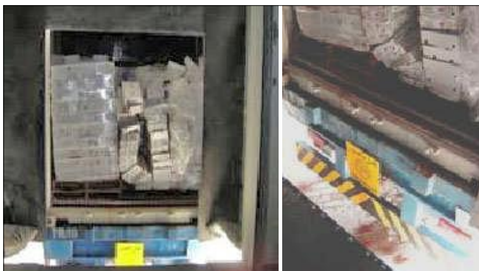
Figure 5. Refrigeration unit failed in the truck transporting frozen meat en route (left). The outside air temperature was 120°F. Blood from thawed meat flowed from the truck when inspectors opened the doors (right).
